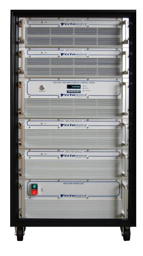
The amplifier can be controlled from either the front panel or remote control via the Ethernet, USB and GPIB interfaces. The digital interface system manages enabling and disabling the amplifier, monitoring power levels, monitoring power supply health, communicating with the control computer and implementing electrical interlocks. The keypad and display interface is used for monitoring amplifier state, power levels, interlock states etc. and for configuration option.
